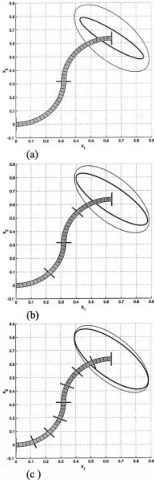
Fig. 7. For a given configuration, adding actuators “fills out” the CME (bold line) so that it approaches the dimension of the GME (thin line).
