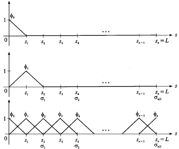
Fig. 5. The first two finite element interpolation functions, followed by all  $n + 1$  functions superimposed.
