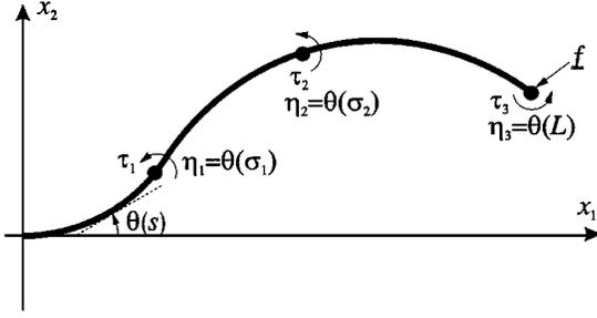
Fig. 3. Three-actuator continuum manipulator with applied end-effector force  $\underline{f}$ .
