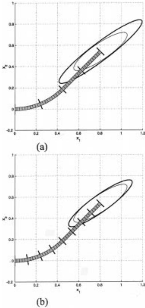
Fig. 8. An illustration of the CFE (bold line) and the GFE (thin line) for two manipulators in the same configuration but with differing numbers of actuators.
