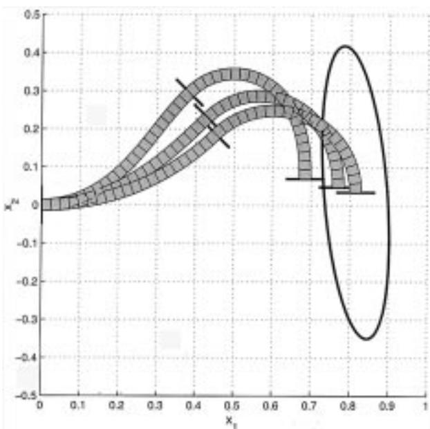
Fig. 10. Forces of the same magnitude as the previous figure encounter relatively less compliance in the horizontal direction.
