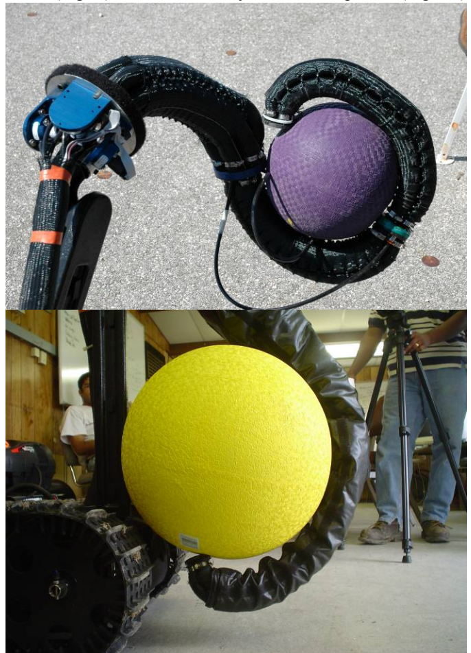
Fig. 11. Grasp of a medium sphere (top). Grasp of a large sphere (bottom).
