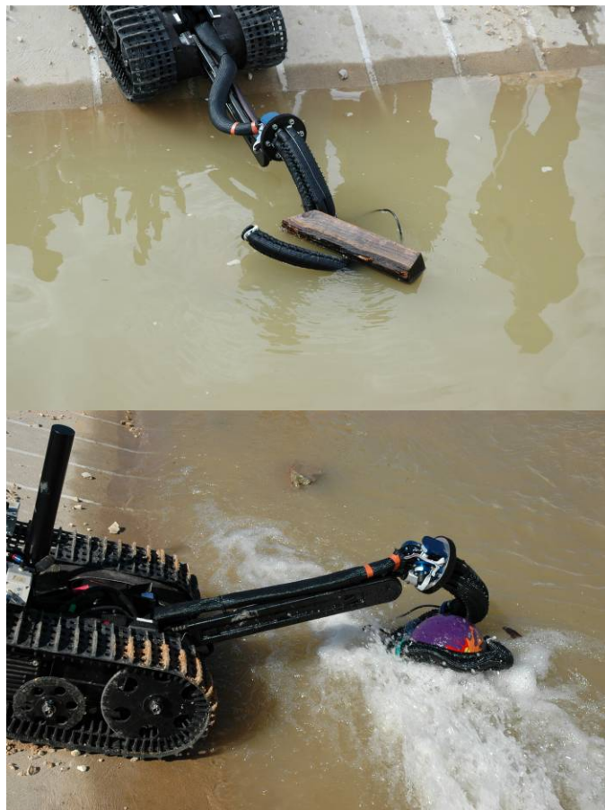
Fig. 12. Grasp of elongated object in water (top). Grasp of medium sphere in water (bottom).
