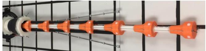
Figure 10. New distal section with emerging Tendril branches
