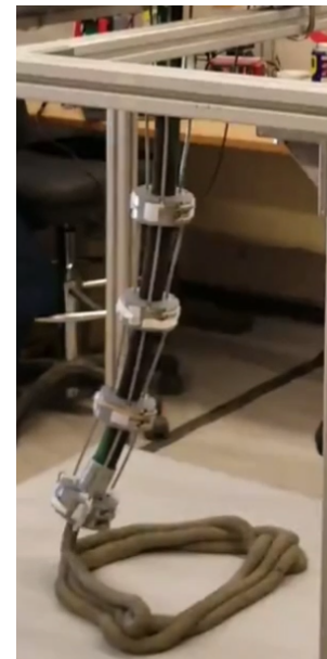
Fig. 8: Concrete printing with cable hose robot
