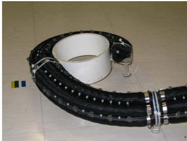
Fig. 1. The Octarm Grasping a Cylindrical Object
