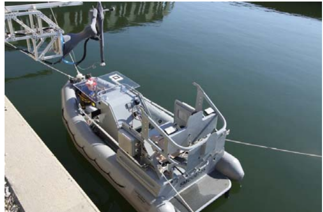
Fig. 7. The US Navy Sea Fox used as the USV in this research at the US Army Aberdeen Test Center wave tank.
