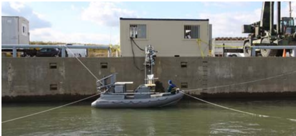
Fig. 10. The US Navy Sea Fox in the ATC wave tank, secured in place to prevent the vessel from moving outside of the test area.
