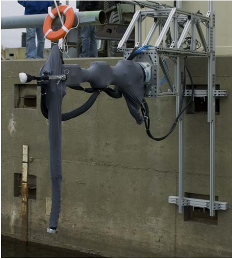
Fig. 9. The truss assembly integrated with the PA10 and Octarm and mounted to the wave tank wall.
