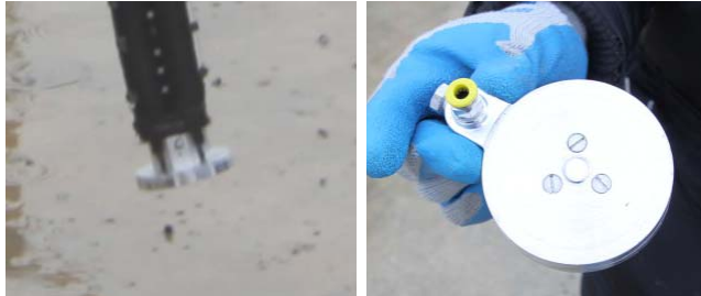
Fig. 5. The magnetic end of the Octarm with the final generation designs of the refueling end effector.
