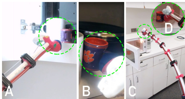
Figure 7: h+lamp collects a cup from the floor and delivers it to a microwave with the user’s cooperation.
